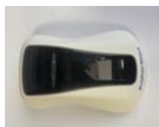
FIGURE 3: Bluephase Meter II for light irradiance monitoring.
