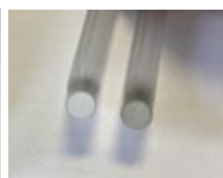
FIGURE 4: Comparison of an old and new light tip.
