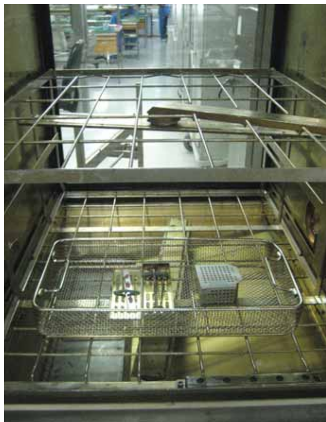
FIGURE 5: Dental instrument test in class 11a washer with hand piece connector.
