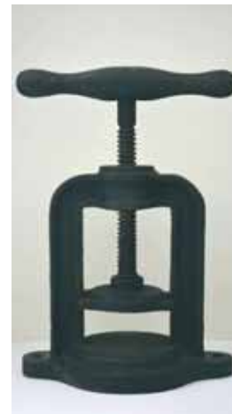
FIGURE 8: A clamp used in the making of vulcanite dentures, c. 1890.
