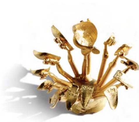
FIGURE 8: The final brackets after investment casting.
