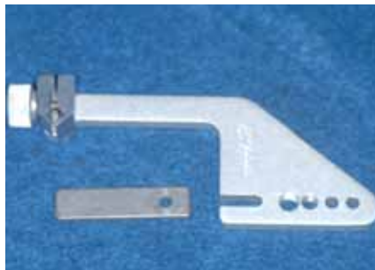
FIGURE 11: Whipmix® mounting jig used to secure the facebow upright in the correct orientation when mounting the maxillary cast. Utilisation of the mounting jig eliminates the need to send the complete facebow to the laboratory; it is only necessary to forward the smaller upright.
