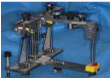
FIGURE 4: Class IV articulator. This is a TMJ highly adjustable articulator.
