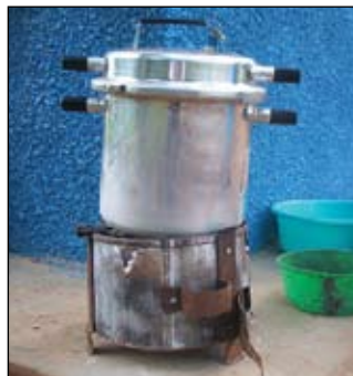
Left: the control measures in place before the team's arrival, and, right, a pressure cooker-type autoclave used by the team.
