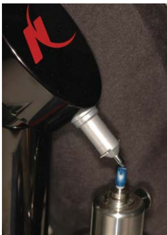
FIGURE 5a: Contact scanner used to scan shape of die or abutment.
