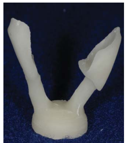
FIGURE 3c: Devested all ceramic pattern replicating wax pattern.
