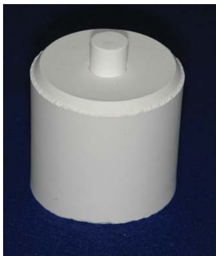
FIGURE 3b: Investment stone with plunger in place after ceramic ingot pressed.
