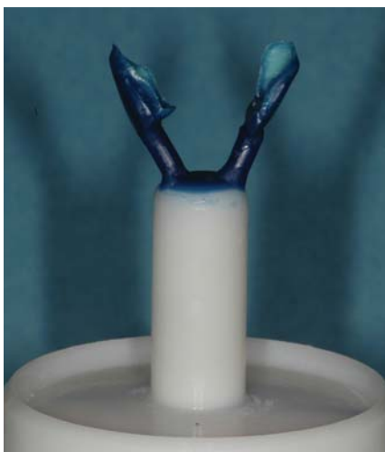
FIGURE 3a: Wax patterns attached to sprue and placed in investing ring before investment poured.
